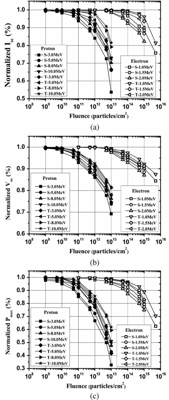
Fig. 1. Normalized parameters (a)  $I_{sc}$ , (b)  $V_{oc}$ , and (c)  $P_{max}$  of the solar cells as a function of electron and proton fluence under different energies. T: Triple-junction cell, S: Single-junction cell.
