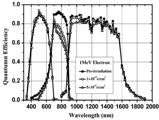
Fig. 2. Electron radiation-induced spectral response degradations of a triple-junction GaInP<sub>2</sub>/GaAs/Ge solar cell.
