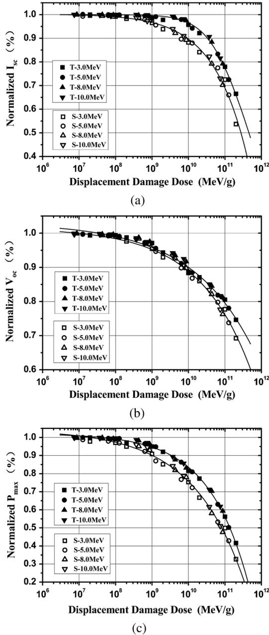
Fig. 4. Normalized parameters (a)  $I_{sc}$ , (b)  $V_{oc}$ , and (c)  $P_{max}$  as a function of proton  $D_d$ . The symbols represent the experimental data and the solid line represents the fitting curve for the cells.
