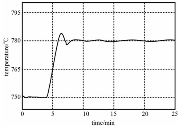
Figure 3 Temperature control curve of resistance-heated furnace
