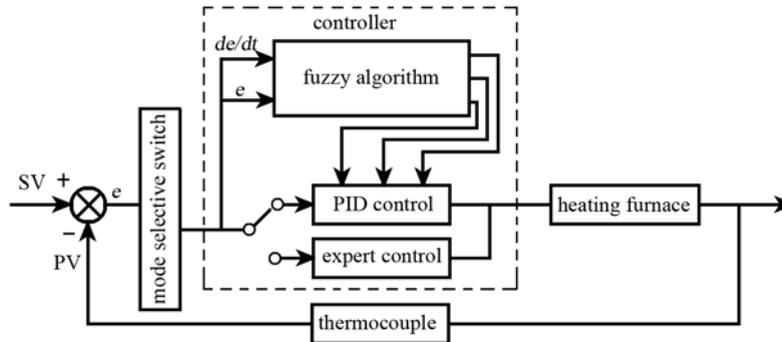
Figure 1 Temperature control system of heating furnace based on expert fuzzy PID
