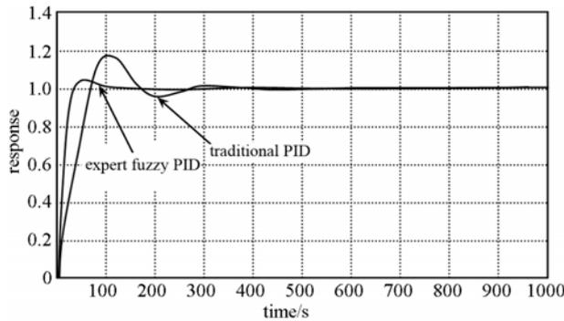
Figure 2 Simulation results of PID and Fuzzy-PID control
