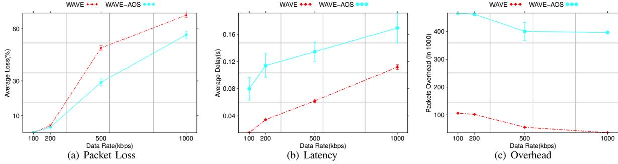
Fig. 1. Experimental Results of WAVE-AOS vs. WAVE approach
