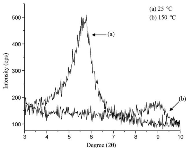
Fig. 3. XRD spectra of the natural MMT at (a) ambient laboratory conditions and (b) after heat treated for 2 h at  $150^\circ\text{C}$ .
