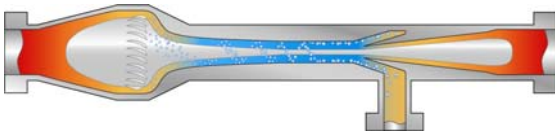
Figure 1: Artist impression of the “Twister Supersonic Separator”. The flow direction is from left to right. The separated liquid and slip gas are transported towards the bottom. The dry gas is continuing to the right.
