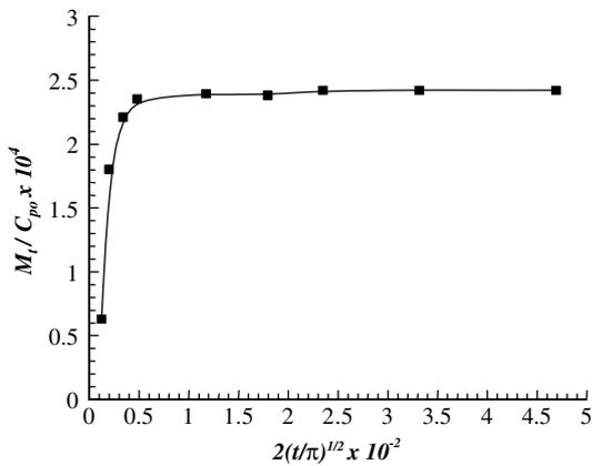
Fig. 3. Plot of  $x = (t/\pi)^{1/2}$  versus  $y = M_t/C_{p0}$  for DEHA from non-irradiated PVC film into isooctane at 20 °C.
