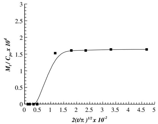
Fig. 5. Plot of  $x = (t/\pi)^{1/2}$  versus  $y = M_t/C_{p0}$  for ATBC from non-irradiated PVC film into isooctane at 20 °C.
