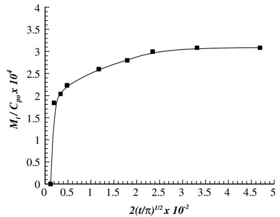
Fig. 6. Plot of  $x = (t/\pi)^{1/2}$  versus  $y = M_t/C_{p0}$  for ATBC from irradiated (25 kGy) PVC film into isooctane at 20 °C.
