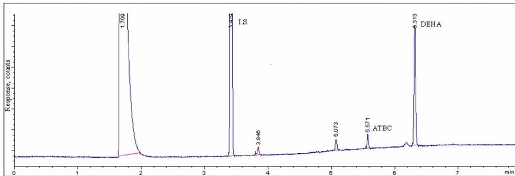
Fig. 2. Gas chromatogram of DEHA and ATBC in irradiated at 25 kGy PVC film into isooctane at 20 °C.
