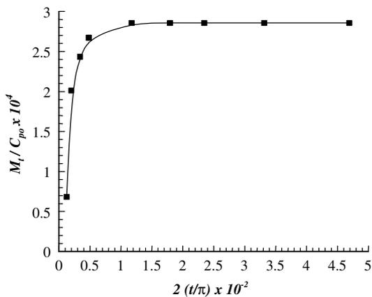
Fig. 4. Plot of  $x = (t/\pi)^{1/2}$  versus  $y = M_t/C_{p0}$  for DEHA from irradiated (25 kGy) PVC film into isooctane at 20 °C.
