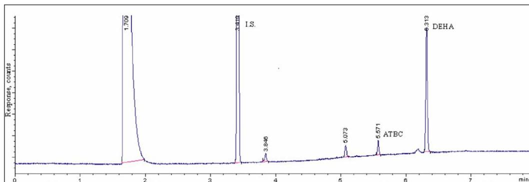
Fig. 1. Gas chromatogram of DEHA and ATBC in non-irradiated PVC film into isooctane at 20 °C.
