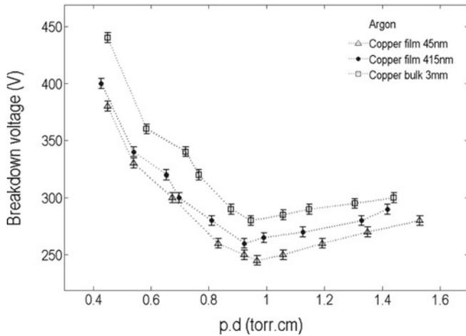
**Fig. 2.** Paschen's curve for argon gas using copper thin films electrodes.
