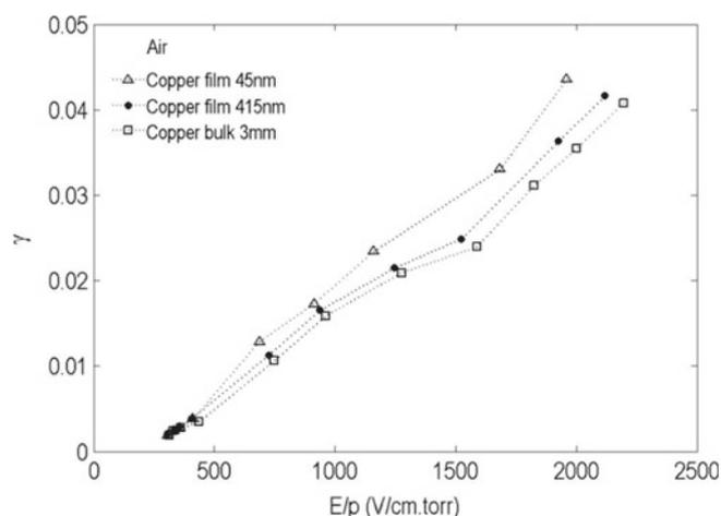
**Fig. 7.** The effective secondary electron emission coefficient  $\gamma$  as a function of the reduced electric field  $E/p$  using copper thin films electrodes for air.
