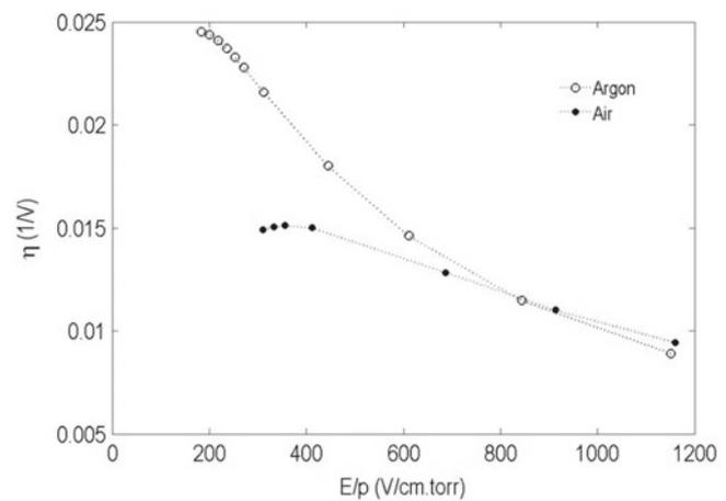
**Fig. 5.** The ionization coefficient as a function of reduced electric field  $E/p$  for air and argon gas.
