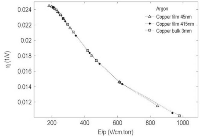
**Fig. 4.** The ionization coefficient as a function of reduced electric field  $E/p$  in the presence of argon for three types of electrodes.
