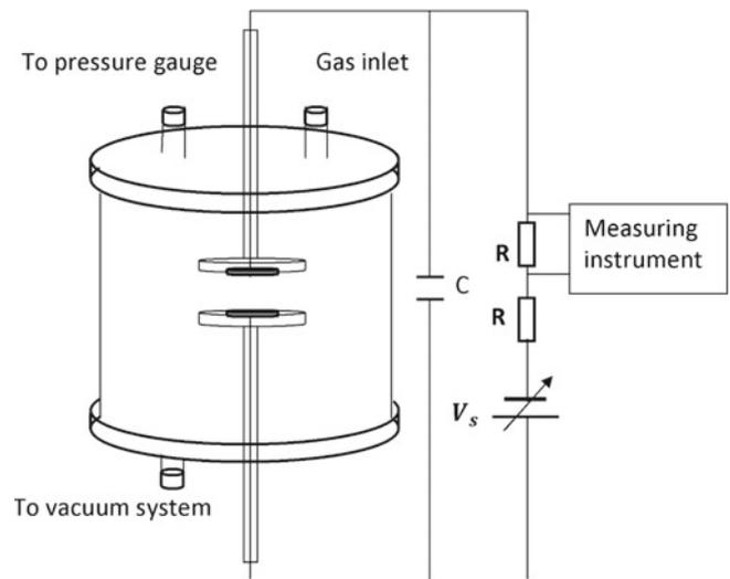
**Fig. 1.** Schematic diagram of the discharge tube and measuring circuit.
