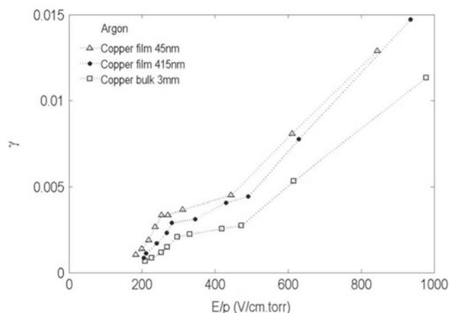
**Fig. 6.** The effective secondary electron emission coefficient  $\gamma$  as a function of the reduced electric field  $E/p$  using copper thin films electrodes for argon gas.
