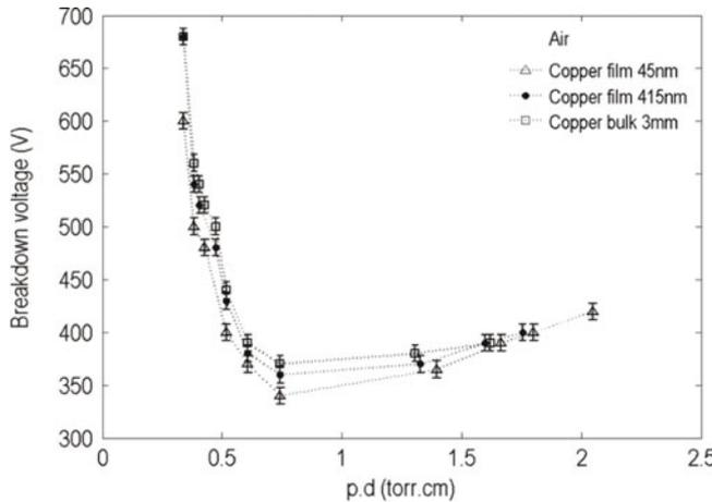
**Fig. 3.** Paschen's curves for air using copper thin films electrodes.
