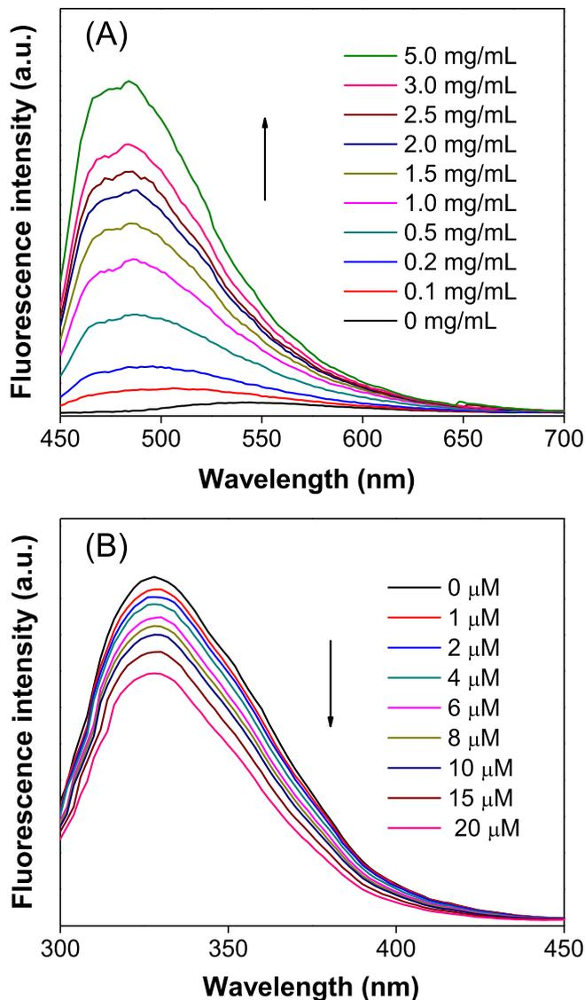
**Fig. 3.** (A) Fluorescence emission spectra of 20  $\mu\text{M}$  curcumin solution at the excitation wavelength of 420 nm in the presence of WPI at different concentrations (0–5.0 mg/mL); (B) Fluorescence emission spectra of 1.0 mg/mL WPI solution at the excitation wavelength of 280 nm in the presence of curcumin at different concentrations (0–20  $\mu\text{M}$ ).
