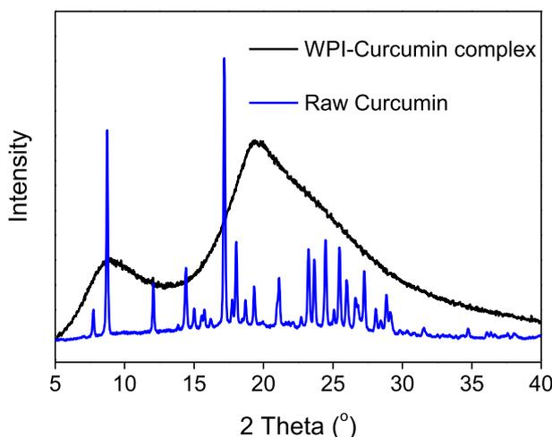
**Fig. 5.** Powder X-ray diffraction patterns of raw curcumin powder and WPI-curcumin microparticles spray dried at 110 °C.
