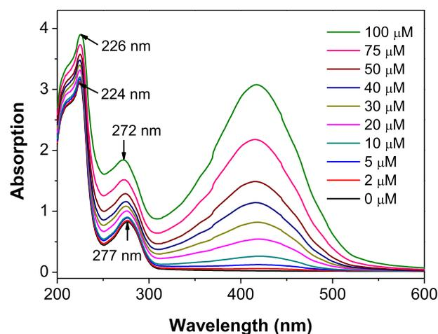
Fig. 2. UV–visible absorption spectra of WPI solutions (1.0 mg/mL) containing different amounts of curcumin (0–100  $\mu\text{M}$ ).
