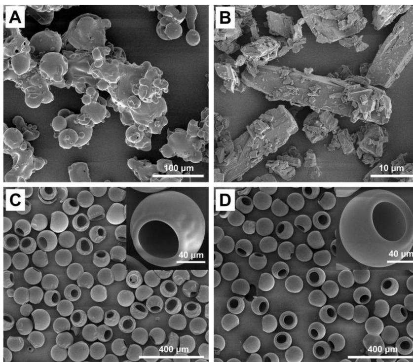
**Fig. 4.** SEM images of (A) raw WPI powder; (B) raw curcumin powder; microparticles of WPI-curcumin complexes spray dried at inlet temperatures of (C) 150 °C and (D) 110 °C.
