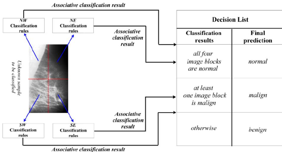
Fig. 6 Decision-making scheme employed to predict the class of unknown samples.
