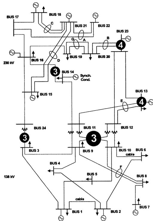
Fig. 5. Interdiction plans 3 (③) and 4 (④) for RTS1 with  $M = 6$  and explicit modeling of system restoration over time. Total energy shed is 557 712 MWh for plan 3. Plan 4 (attack to two buses) is created assuming the two substations attacked in plan 3 have been rendered invulnerable. Total energy shed drops to 272 160 MWh.
