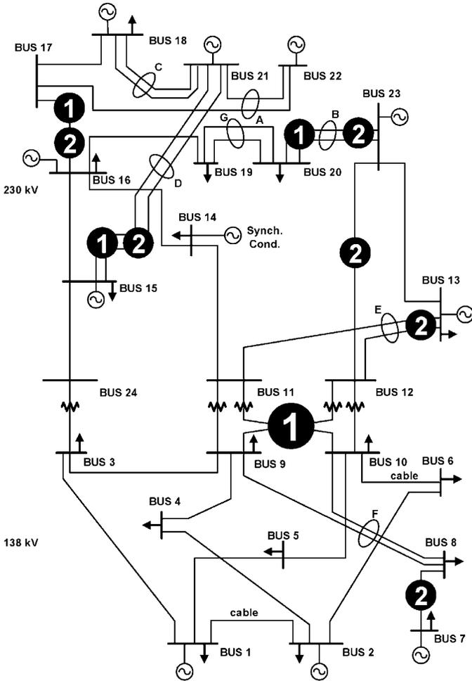
Fig. 3. Two interdiction plans (depicted as ① and ②) for RTS1 using  $M = 6$ . Total load is 2850 MW. Plan 1 sheds 1258 MW and plan 2 sheds 1373 MW. The large “①” indicates that the four transformers and buses in the substation are interdicted.
