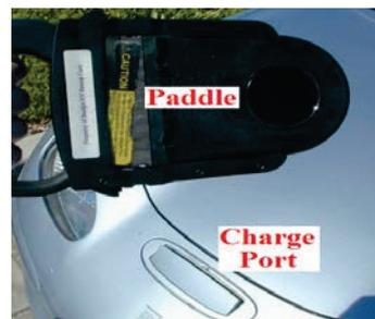
Fig. 3. Typical inductively coupling stationary EV battery charging and GM EV1 system.
