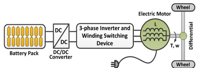
Fig. 2. Typical structure of integrated EV charger.
