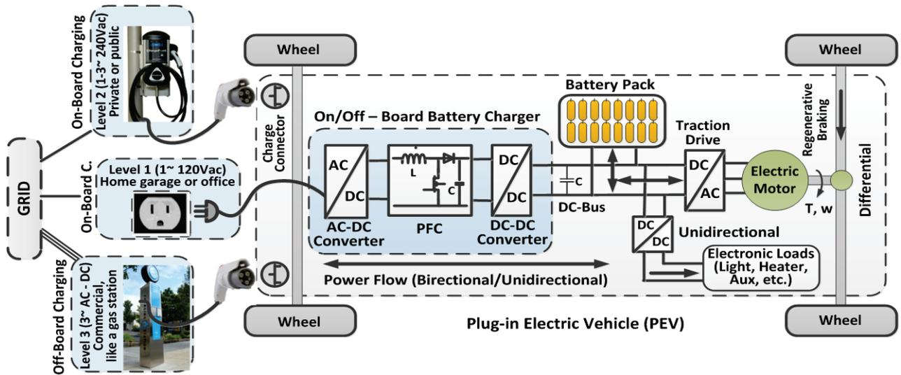
Fig. 1. On/off board plug-in electric vehicle charging system and power levels.
