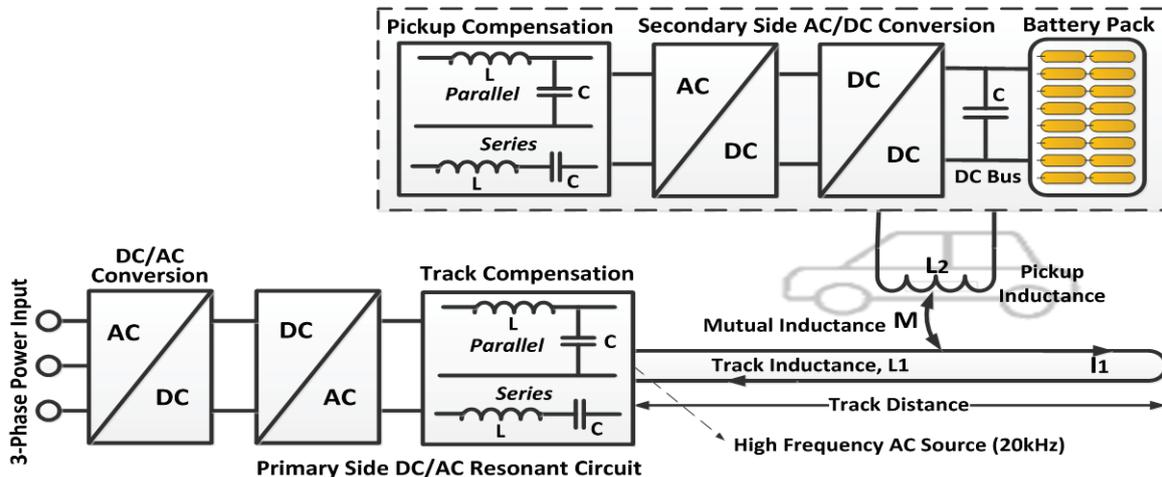
Fig. 4. Inductively coupling roadbed EV battery charging system
